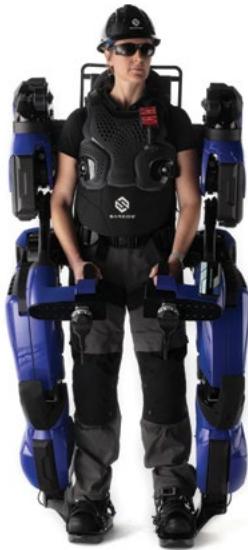
FIGURE 7.6 Sarcos Guardian XO Max wearable exoskeleton
